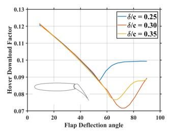
Figure 13.1: Hover download as a percentage of gross weight for various flap configurations in hover
