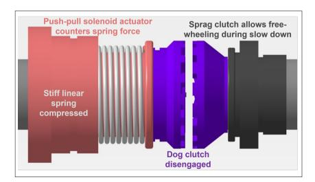
Figure 10.5: Internal view of the Terp Two-Speed Transmission clutch system when Arion is in hover mode.
