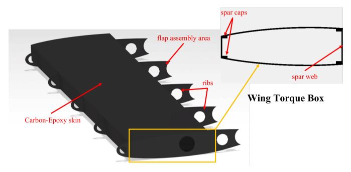
Figure 8.5: The primary load-bearing structure of the wing (shown without flaps / flaperons)
