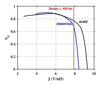
Figure 13.7:  $\eta_p$  versus propeller advance ratio
