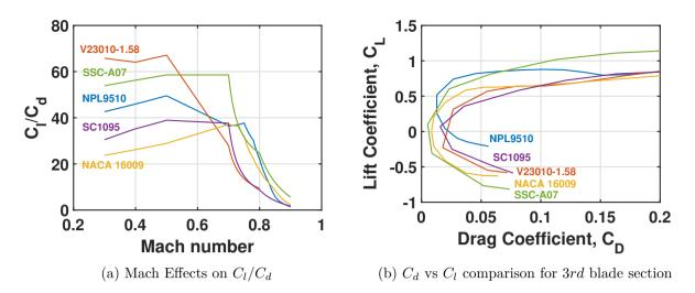
Figure 5.7: In-house CFD predicted Characteristics of best aerodynamic performance airfoils
