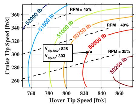
Figure 5.10: Gross takeoff weight [lb] variation with hover and cruise tip speeds
