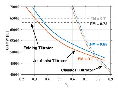
Figure 4.3: Predicted Gross Take-off Weight versus propulsive efficiency for folding and jet-assist tiltrotor
