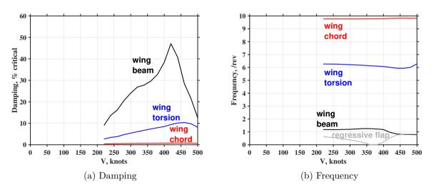
Figure 6.7: Whirl flutter stability analysis of coupled modes at 27,000 ft
