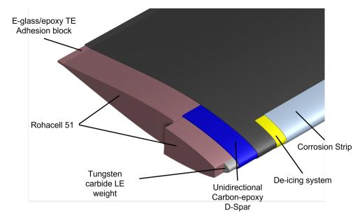
Figure 6.1: Blade internal anatomy with materials
