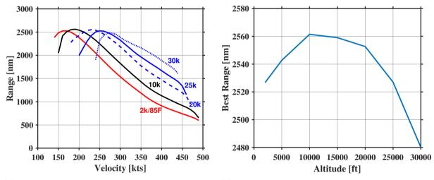
(a) Range vs. Velocity with 20 minutes reserves at (b) Maximum range vs. altitude with 20 minutes several altitudes reserves in mission conditions: atmospheric ISA, ground at 2k/85°F
