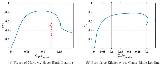
Figure 5.2: Effect of blade loading on hover and cruise performance
