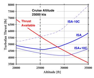
Figure 13.5: Turbofan Thrust 450 kt cruise.
