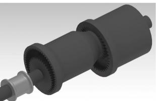
a 2-stage gear set and a planetary gear.
