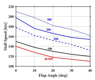
Figure 8.3: Stall Speed Varying with Flap Deflection at Different Altitudes and ISA conditions
