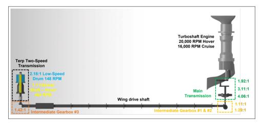
Figure 10.3: Final powertrain layout.
