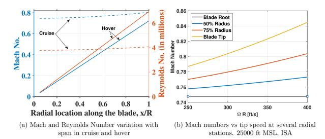
Figure 5.4: Mach and Re Number variation with span and tip speed
