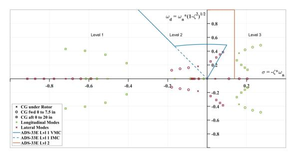
longitudinal oscillation dynamics resulting in shortened time to double. Handling the aircraft under these conditions would result in a high workload and the inability to perform additional tasks for the pilot.
