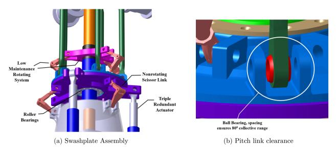
Figure 7.2: In-depth component details of the hub and swashplate assemblies
