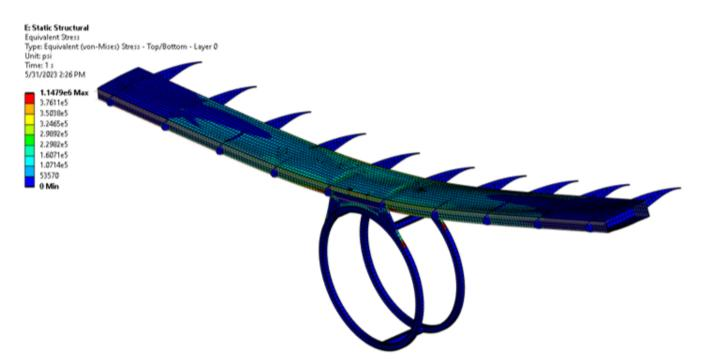
Figure 8.6: Finite element analysis of the wing-fuselage connection
