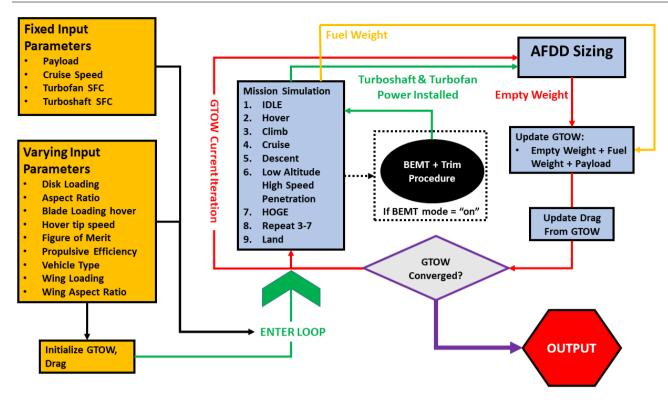
Figure 4.2: Flowchart for the configuration sizing procedure
