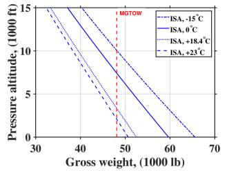
Figure 13.4: Maximum HOGE altitude vs. GTOW for various of ISA conditions
