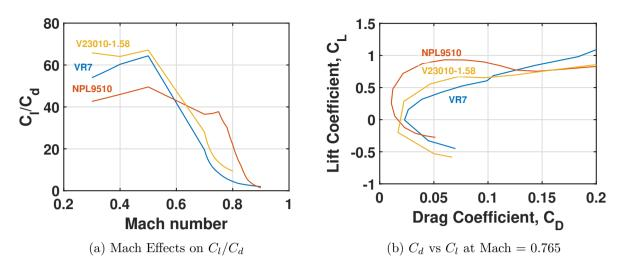
Figure 5.6: In-house CFD predicted performance of airfoils in the transition region
