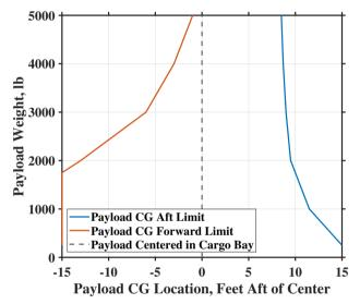
Figure 14.1: Allowable range of payload CG relative to the cargo bay center based on CG analysis with zero fuel weight.
