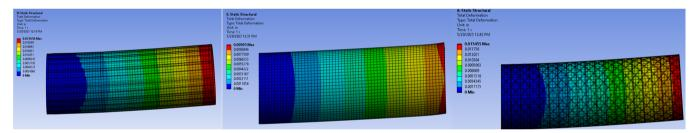
Figure 9.3: Finite element displacement for each of the fuselage designs. From left to right the conventional aluminum fuselage, conventional composite fuselage and geodesic fuselage
