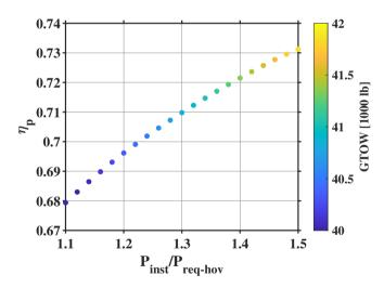
Figure 5.18: Cruise propulsive efficiency variation with turboshaft power installed. Colors indicate the resulting design GTOW.
