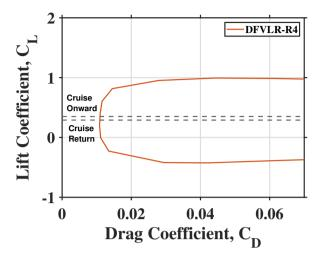
Figure 8.2:  $C_d$  vs  $C_l$  at cruise speed with  $11^{\circ}$  sweep
