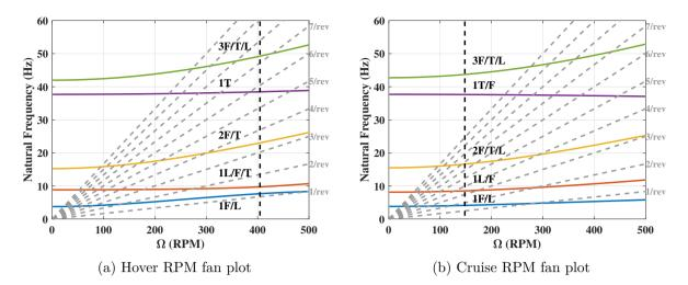
Figure 6.3: Fan plots showing first five rotor frequencies at hover and cruise RPM
