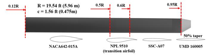
Figure 5.19: Final blade aerodynamics design
