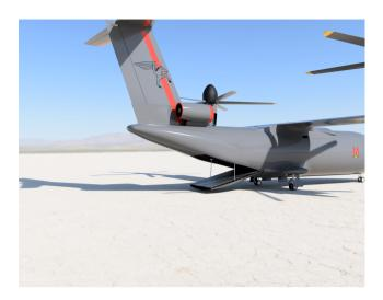
Figure 9.5: Rear cargo ramp open for loading cargo, vehicles, or personnel
