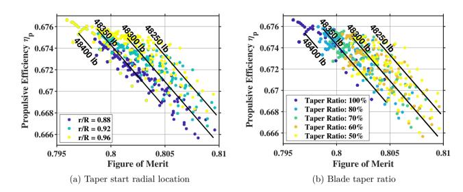
Figure 5.14: Linear taper characteristics effect on vehicle design
