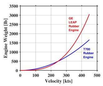
Figure 4.4: Turboshaft and turbofan weights required to overcome drag of a vehicle with a flat plate area of 11.5  $ft^2$
