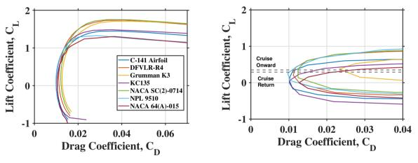
(a)  $C_d$  vs  $C_l$  at forward speed of Mach 0.3 (b)  $C_d$  vs  $C_l$  at cruise speed with no wing sweep
