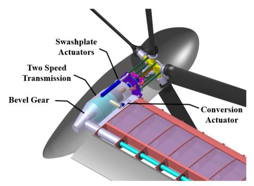
Figure 8.7: Pylon Interior shown in Axial Flight
