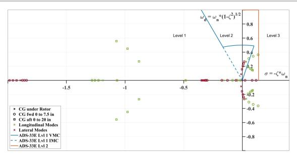
Figure 15.3: Hover Stability Modes with Pitch, Roll, and Yaw Rate Electronic Feedback Damping. Red symbols are the longitudinal modes, and blue symbols are the lateral-directional modes. Squares reflect CG shifting forward up to 7.5 inches (19 cm) from the rotor shaft. Circles reflect the CG shifting aft up to 20 inches (51 cm) from the rotor shaft.
