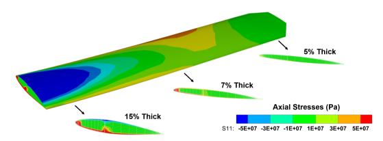
Figure 6.8: Axial stress distribution of Arion blade in hover,  $C_T/\sigma = 0.12$ .
