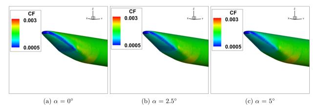
Figure 12.8: Fuselage skin friction coefficient distribution in ramp region for different body pitch angles
