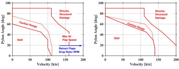
(a) Normal conversion corridor for Arion shows (b) Conversion corridor without flaps. A safe no-flap plenty of margin and a clear path to convert to forward flight.
