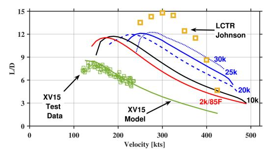
Figure 13.6: L/D vs. Velocity. ISA conditions within RFP requirement of 20k ft (6,096 m) or greater (blue), 10k ft (3,048 m), ISA (black), and 2k/85°F (red) are displayed. Flight test data from XV15 along with the analytical model, and LCTR analytical predictions are also shown [1]
