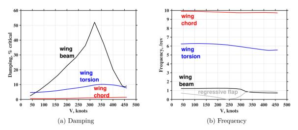
Figure 6.6: Whirl flutter stability analysis of coupled modes at 2000 ft
