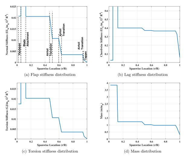
Figure 6.2: Rotor Blade Sectional Properties
