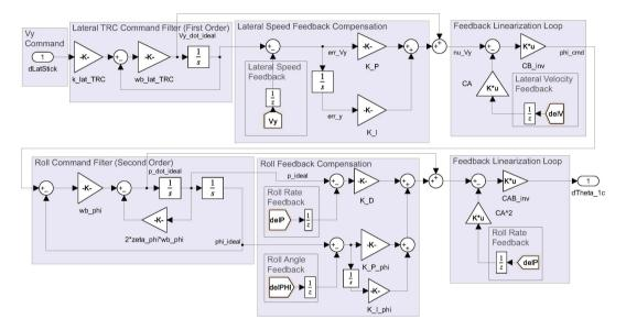
Figure 15.4: Example of TRC DI Inversion for Lateral Stick Inputs in a Hover
