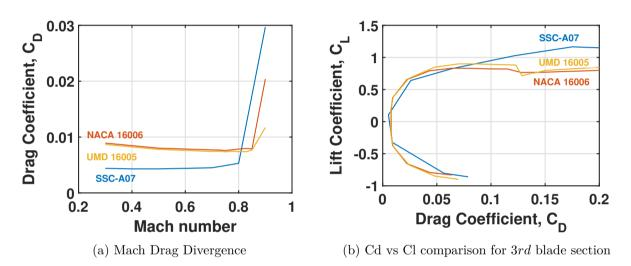
Figure 5.8: In-house CFD predicted Characteristics of best aerodynamic performance airfoils
