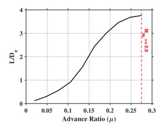
Figure 13.13: Rotor Lift-to-drag ratio  $(L/D_e)$  variation with advance ratio. Flight beyond an advance ratio  $\mu = 0.275$  is restricted by the VMS to prevent shocks over the rotor blade
