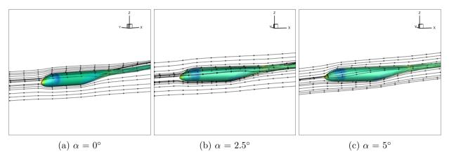
Figure 12.7: Fuselage pressure distribution and flowlines for different body pitch angles
