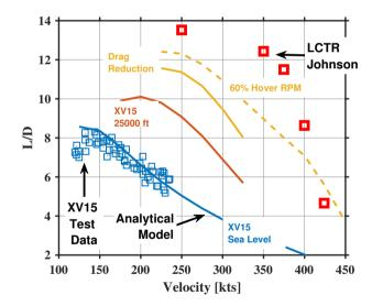
Figure 5.3: L/D vs velocity for modified XV-15 with test data (conceptual study)
