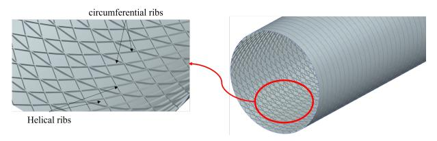
Figure 9.2: Geodesic fuselage geometry and design
