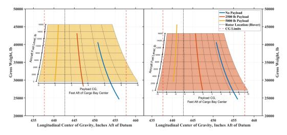
Figure 14.2: Aircraft CG variation within the allowable range due to payload weight (left is 5,000 lb and right is 2,500 lb), payload CG location within cargo bay (sub-axis abscissa), and aircraft fuel level (sub-axis ordinate).
