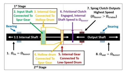
Figure 10.1: Simplified diagram of the NASA offset compound gear in hover mode.
