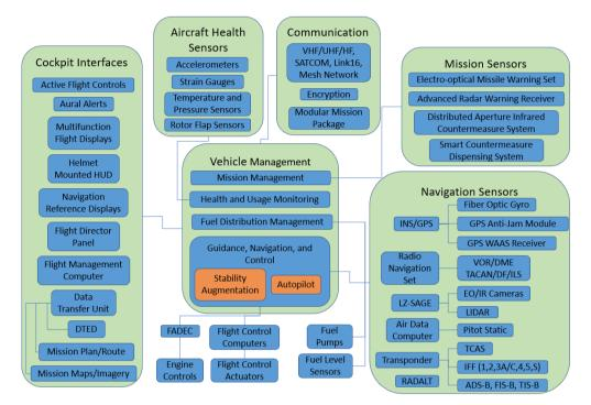
Figure 16.1: Avionics architecture of Arion
