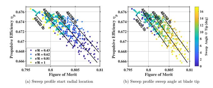
Figure 5.13: Scimitar sweep profile characteristics effect on vehicle design
