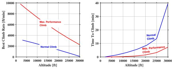
(a) Best Climb Rate in feet per minute versus al- (b) Time to climb in feet per minute versus cruise titude in atmospheric ISA conditions, where ground is at  $2k/85^{\circ}F$
