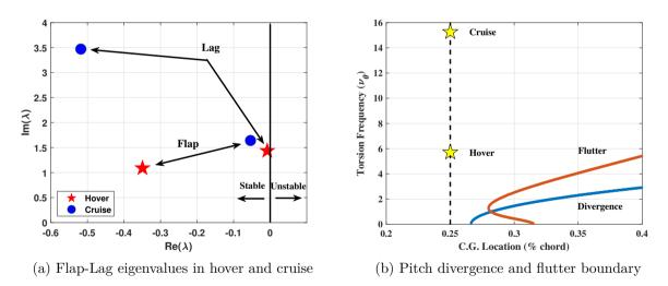
Figure 6.5: Flap-lag and pitch-flap stability margins
