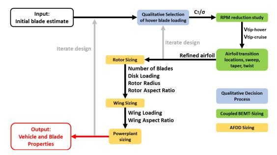
Figure 5.1: Vehicle Sizing and Aerodynamic Design Process
