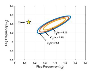
Figure 6.4: Flap-lag flutter boundaries at  $\theta_{tw} = -21^{\circ}$ with increasing blade loading
