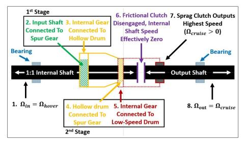
angular rate for cruise as shown by marking 8 in Figure 10.2.
