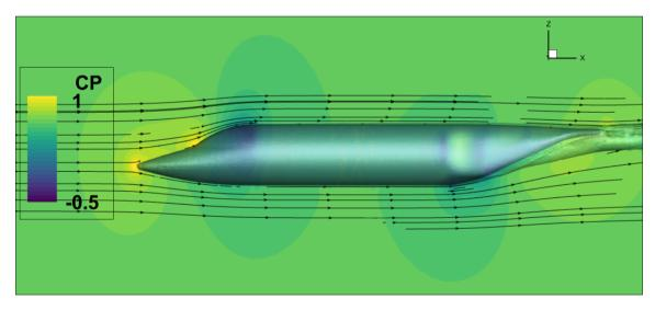
Figure 12.1: Fuselage Version 1.0 Pressure Distribution
