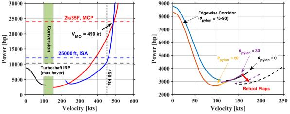
(a) Power vs. velocity at 25,000ft/ISA and 2k/85°F (b) Power versus velocity during conversion. Solid lines: 40 degrees of flaps, Dashed lines: 0 degrees of flaps
