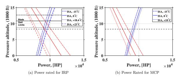
Figure 13.3: HOGE power required (blue) and power available (red) for various ISA conditions
