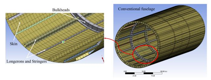
Figure 9.1: Semi-monocoque architecture for metal and composite primary airframe structure showing the basic load-bearing elements.
