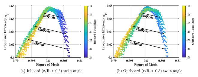
Figure 5.15: Blade bilinear twist selection
