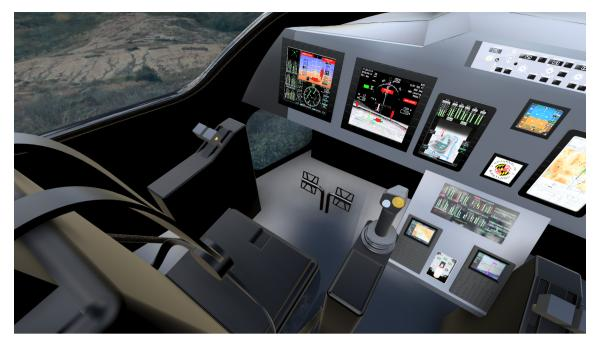
Figure 15.1: Cockpit controls including active side stick, split-power thrust control lever, and foot pedals.
