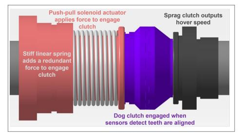
Figure 10.6: Internal view of the Terp Two-speed Transmission clutch system when Arion is in cruise mode.
